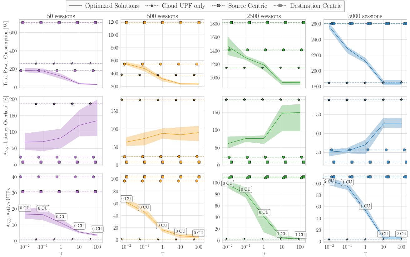
Fig. 10: Optimized UPF selection and three heuristic baselines evaluated across session volumes at varying energy weight \gamma . The first row reports aggregate power drawn by all active UPFs. The second row reports average latency overhead relative to an ideal zero-load reference, where all UPFs are available and unloaded. The third row shows the average number of active UPFs, with active cloud UPF (CU) counts annotated per panel. Horizontal dashed lines mark heuristic solutions, whose performance is invariant to \gamma . Note the different y-axis scales across plots.
